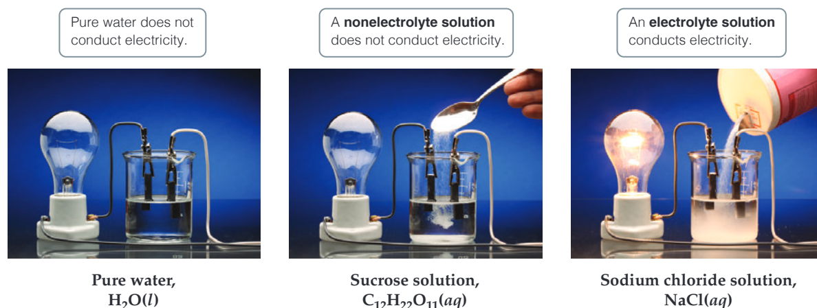
▲ Figure 4.1 Completion of an electrical circuit with an electrolyte turns on the light.
